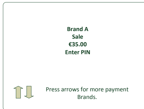
Figure 9: EXAMPLE 5 (STEP 1): CONTACT - ACCEPTOR PREFERRED SELECTION WITH OVERRIDE ON THE SAME SCREEN USING ARROWS
